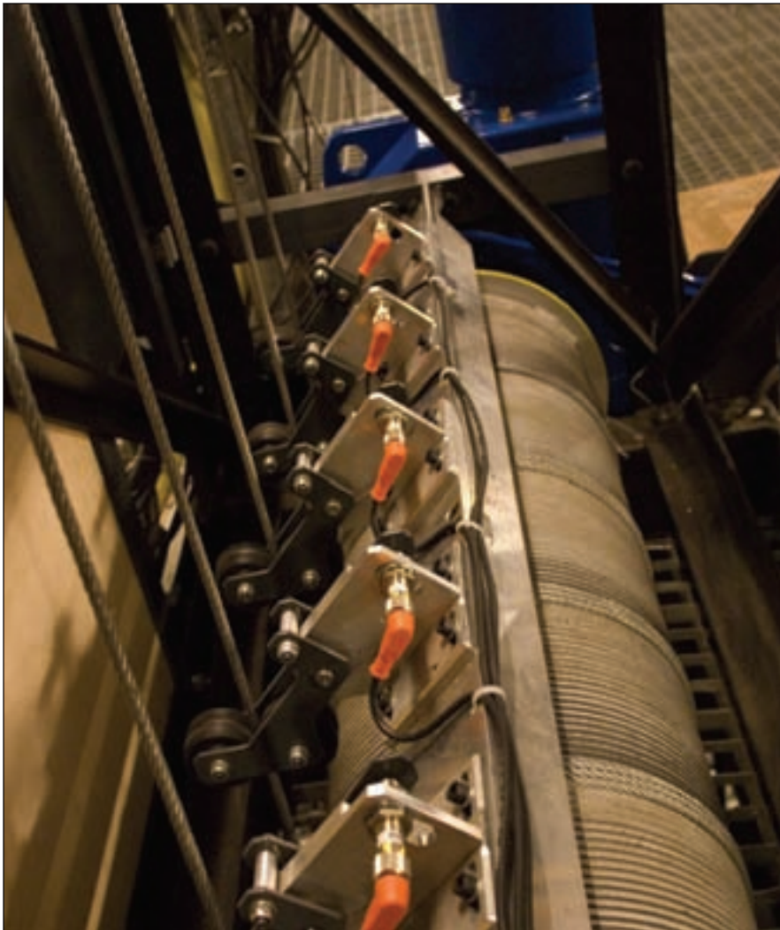
New slack wire detection was installed to increase safety (courtesy of Sprint Electric).
