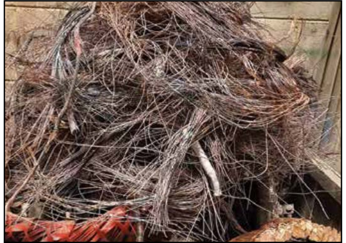
Figure 1 Typical copper scrap after motor burnout at EECO.
