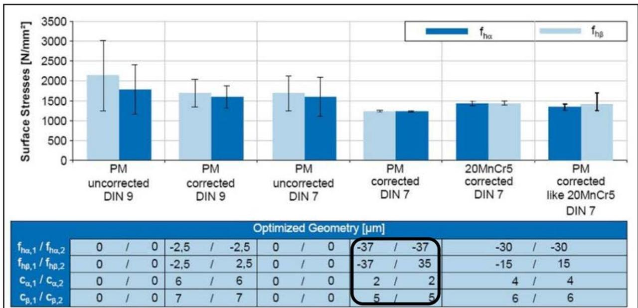
Figure 2 Surface stress of PM with different modifications.
