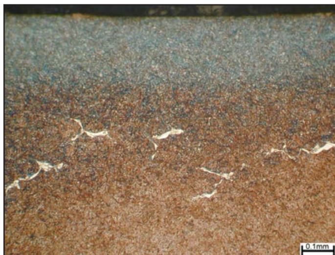
Figure 11 irWEAs on rotor bearing ROT-D IR.
