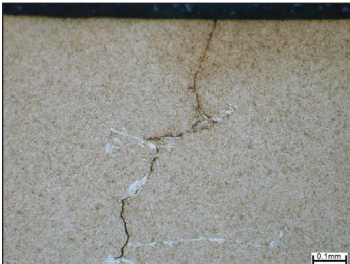
Figure 3 Irregular white etching areas on axial crack.
