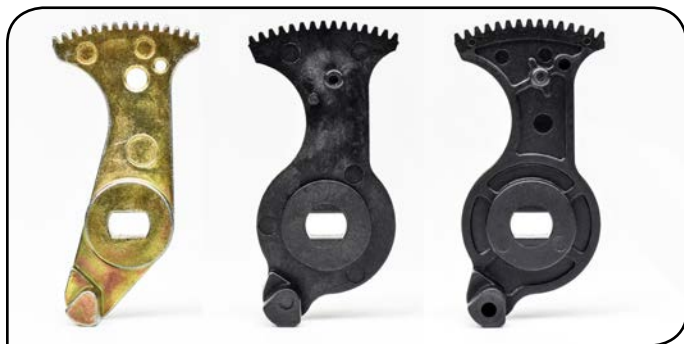
Figure 1 Zinc gear International Plastics prototyped, followed by first production gear (All photos courtesy International Plastics LLC).
