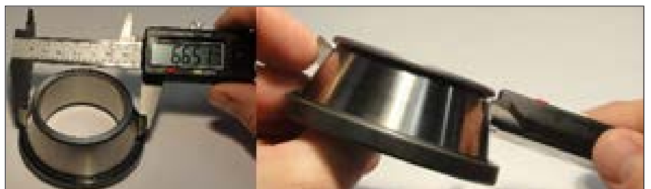
Figure 2 Measuring major and minor inner raceway diameters for D_{pw} .
