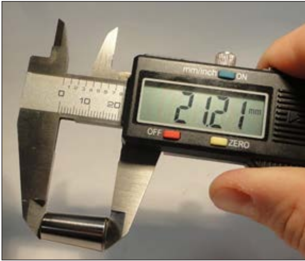
Figure 3 Measuring roller length for L_{we} .
