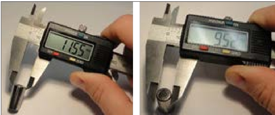
Figure 4 Measuring roller ends for D_{we} .
