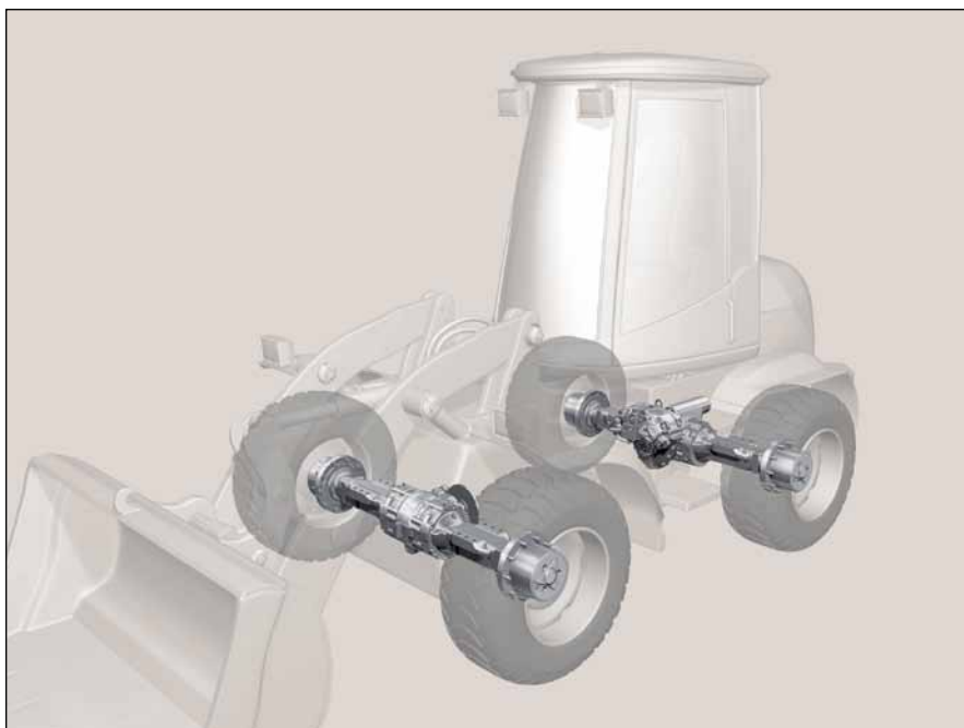
ZF has met the increasing demands of lower fuel consumption in compact loaders with its hydrostatic drive technology (courtesy of ZF).
