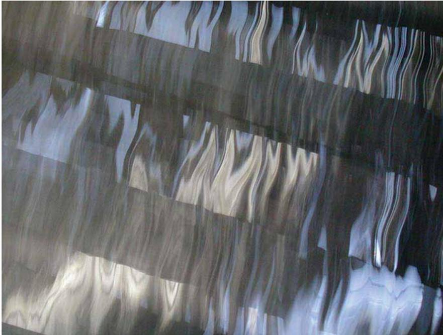
**Figure 6—Properly lubricated open gear.**
