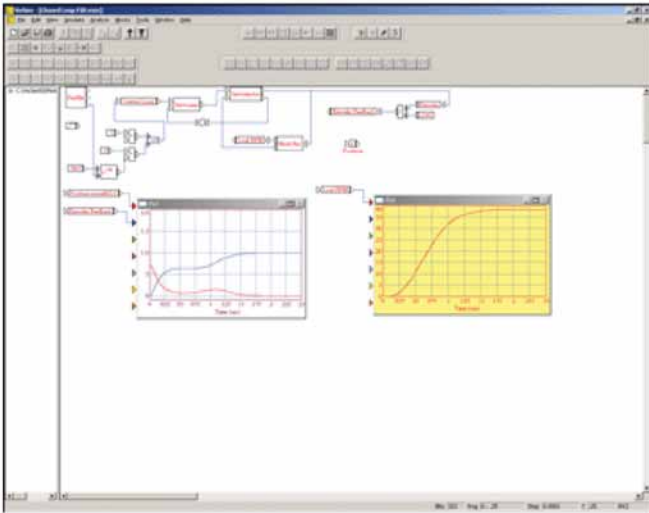
Figure 2—Simulation illustrating a screen shot of a block functional diagram of a closed-loop system. The left-hand graph depicts the position error in red and the encoder feedback in black. The load speed (rpm) vs. time is shown in the right-hand graph. The result of different gain, acceleration and velocity constants can be seen as they are changed.
