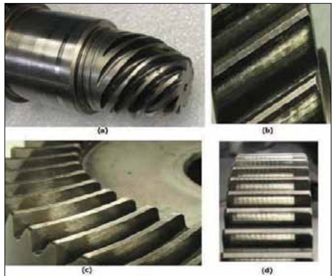
Figure 7—Hyponic gear components after 2.5 million cycles: a) hypoid pinion; b) spur gear; c) hypoid gear; d) spur gear pinion (Ref. 2).
