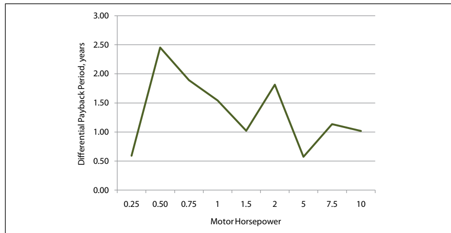
Figure 2—Calculated differential payback period by motor horsepower, based on average purchase price from distributor.
