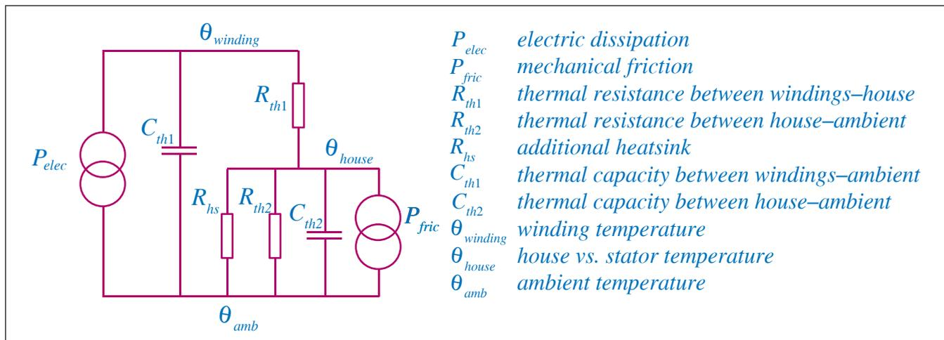
Figure 2—Detailed thermal model for PM (Permanent Magnet) motor.
