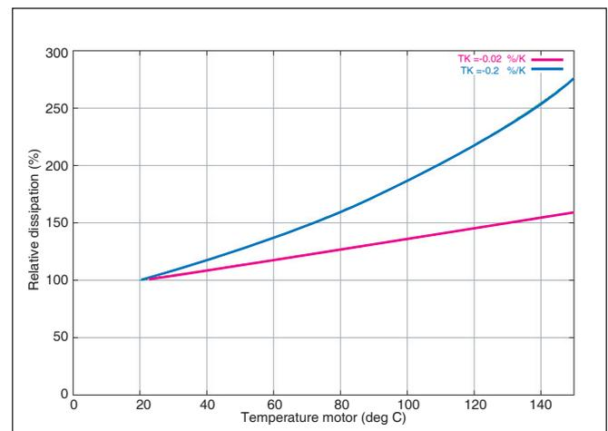
Figure 1—Dissipation increases at increasing motor temperature.
