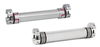
jaws from solid round bar stock, precision elastomer couplings hubs possess natural balance and strength beyond those of traditional jaw couplings, allowing the limits for speed and torque within a given size to be increased. They also make use of calibrated polyurethane spider inserts, which are preloaded between the curved jaws. While the curvature increases surface area contact between the jaw and the insert over a shorter distance, increasing torque-density, the preload eliminates
