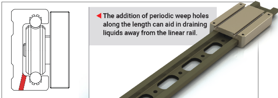
Figure 9— The addition of periodic weep holes can aid in draining liquids away from a linear rail.
