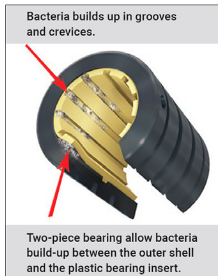
Figure 1 — Bacteria tends to build up in areas that are difficult to clean, such as grooves, crevices, and between the outer shell and plastic insert of two-piece bearings.
