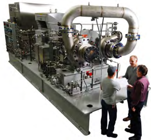
In addition to the traditional refinery/EPI applications, Sundyne also showcased its diaphragm compressors, which are widely used for Hydrogen processing applications.
