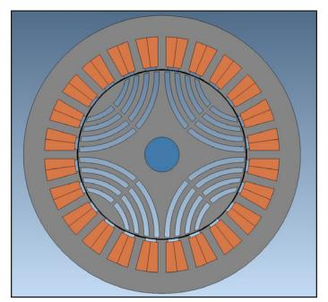
Figure 7 Lamination of the SYR motor.
