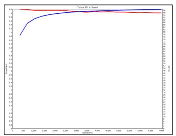
Figure 10 Speed torque of SYR motor.
