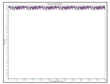
Figure 11 The torque ripple of a SYR motor.
