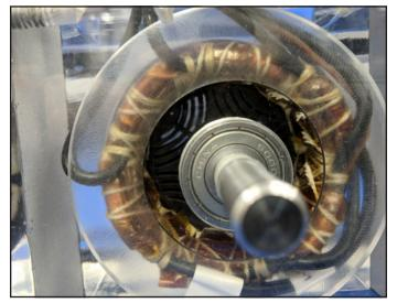
Figure 9 Synchronous reluctance test motor.
