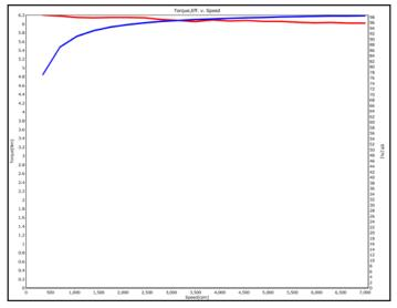
Figure 4 Speed/torque curve of a VSR motor.
