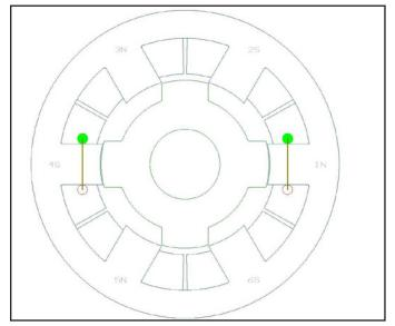
Figure 1 Basic lamination design of a VSR motor.
