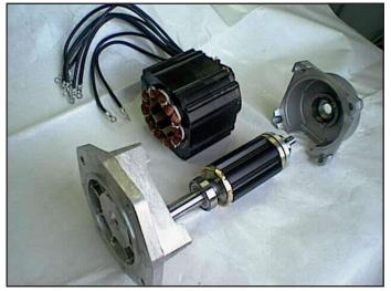
Figure 2 Key components of the VSR motor.
