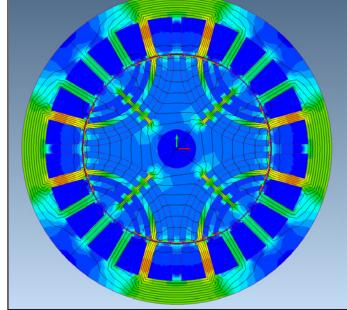
Figure 8 Flux distribution of typical SYR motor.
