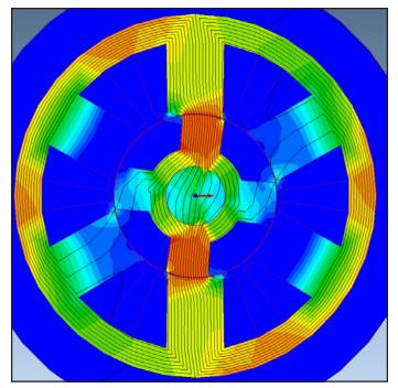
Figure 5 Flux distribution of a typical VSR motor.
