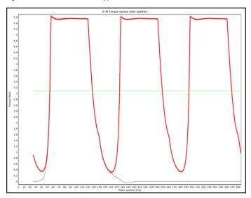
Figure 6 Torque ripple of the VSR motor.
