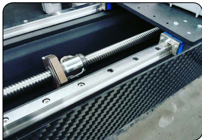
Figure 2 Thomson precision ball screws assist the gantry in moving smoothly and accurately along the X and Y axes.
