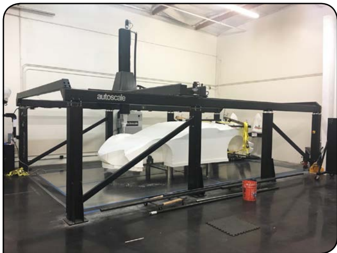
Figure 1 Autoscale's high-performance CNC technology can cut objects up to 16 feet long.
