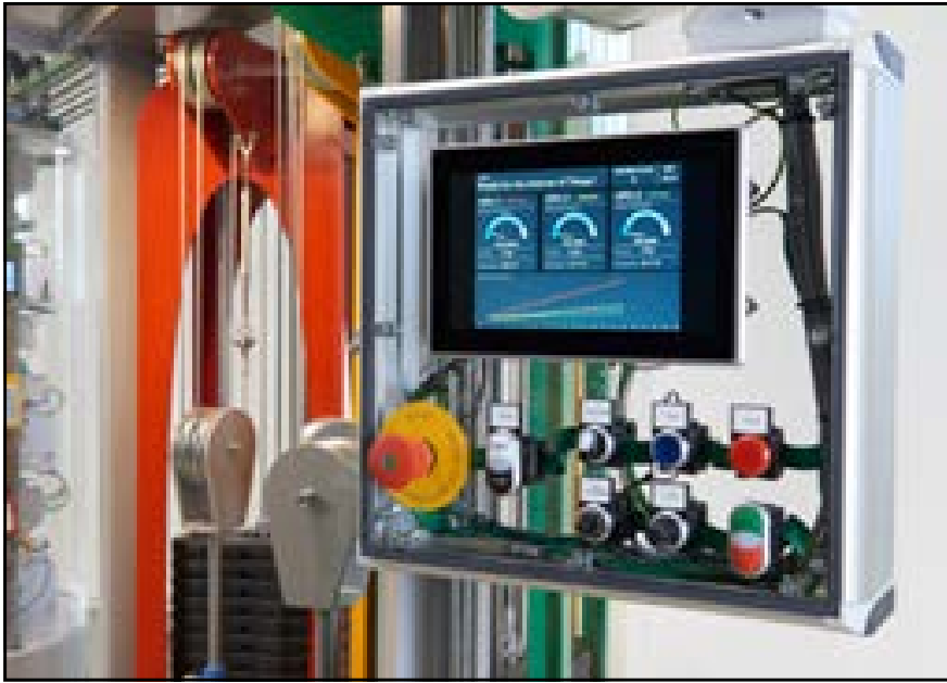
Figure 2 Through integration of an intelligent wiring and communication system, the hydraulic power unit is already IoT-ready, meaning that mechanical engineers and end users can, regardless of location, obtain an up-to-date, detailed overview of all relevant data, such as temperature and pressure.
