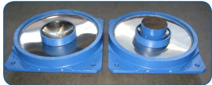
damage a building, the bearings allow the building's foundation to physically move back and forth like a pendulum, finding an outlet to expend otherwise damaging levels of force.
