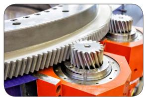
Until now, these constraints meant that manufacturers had to use drives that were generally complex and did not necessarily meet every technical requirement. Redex offers two complementary integrated drives for tables used on milling machines and vertical lathes. They allow designers to choose the right drive for each application and
