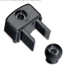
Also available are EN 450.1 plastic spacers for ball-shaped door catches, made of glass fiber reinforced plastic. In addition to the basic spacing distances of 5, 10 and 15 millimeters, combinations of spacers can provide distances of 20, 25 and 30 millimeters as well.
