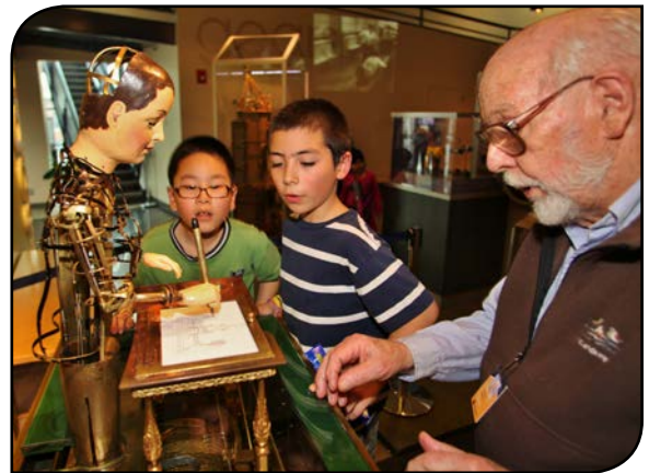
Henri Maillardet’s automaton contains a total of 72 operating cams that control the movements of the right hand. Additional and far simpler cams move the left hand, head and eyes of the doll (photo courtesy The Franklin Institute).
