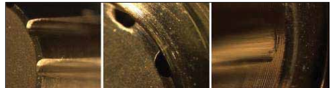
Figure 17—Passed pressing trial results with 40 µm oversize.
