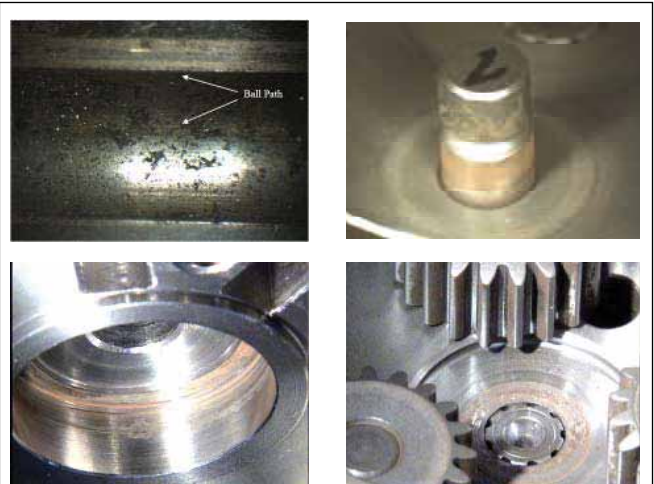
Figure 3—Lubrication failure of first actuator after life test. Visible corrosion results from the exposure of the blank metal to air after disassembly of the actuator.
