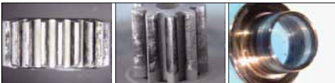
Figure 14—Lead-coated gearbox and lead-bronze bushing after life test.
