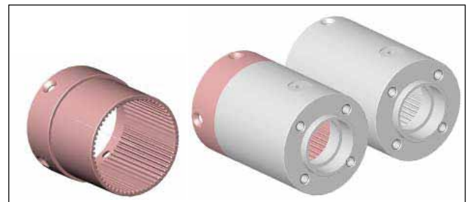
Figure 18—Hollow-wheel ring and integrated design versus gearbox housing made entirely of Cronidur.
