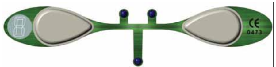
This MSI sensor is embedded in a sleep apnea patch used for monitoring airway flow during sleep. It features strain gage sensing of chest movement, contact microphone-sensing for snoring and pyroelectric sensing for exhalation monitoring (photo courtesy MSI).
