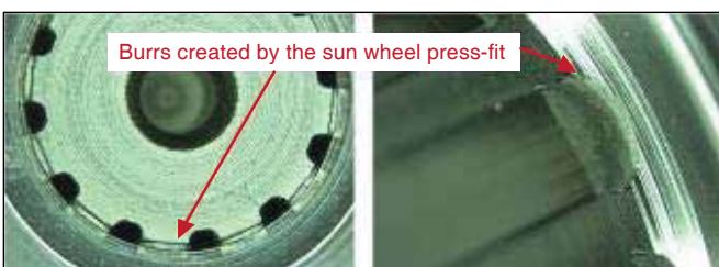
Figure 16—Failed pressing trial results.
