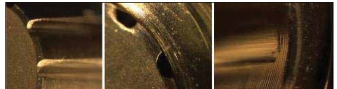
Figure 17—Passed pressing trial results with 40 μm oversize.
