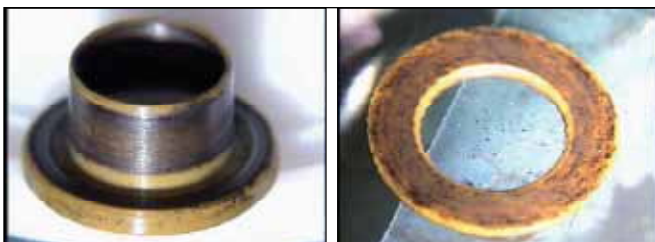
Figure 13: Pre-QM1 Torlon bushing and distance washer after life test.
