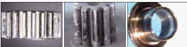
Figure 14—Lead-coated gearbox and lead-bronze bushing after life test.
