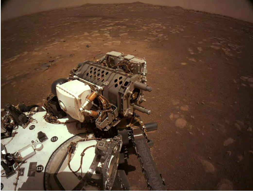
This image shows parts of the robotic arm on NASA's Perseverance rover flexing and turning during its first checkout after landing on Mars. Photo courtesy of NASA/JPL-Caltech.
