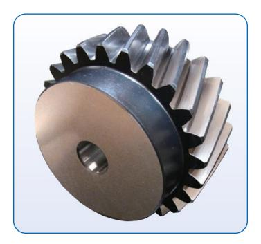
the gradual change to the contact surface load which give helical gears their characteristic of smooth transmission of rotation. Consequently, compared to spur gears, helical gears generate less vibration and noise and perform better in high-speed rotation and high-load applications.
