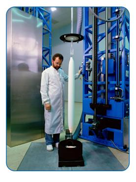
arrives at the heating element, gravity takes over, and the molten silicon drips and narrows to its intended diameter. As it cools and hardens, the filament passes through a laser micrometer to
