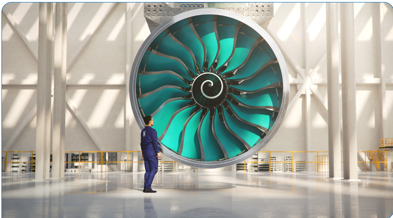
The UltraFan uses a power gearbox—introduced between the fan and intermediate pressure compressor—to ensure that the fan, compressors and turbines all continue to run at their optimum speed.
