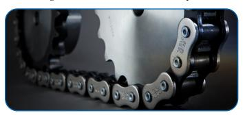
Perhaps the most obvious feature of Tsubaki Titan chain is the use of seamless bushes that incorporate Lube Grooves. The bushes are precision made and perfectly cylindrical, to ensure the smoothest possible operation which in itself will help minimize wear. Enhancing this, the special Lube Grooves ensure oil is retained at the very point of contact—where the chain needs it most. This limits the wear between pin and bush, significantly improving the wear life as a result.
