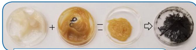
Compatible greases (top) will appear similar after several hours of operation whereas incompatible blends (bottom) can result in darkening of the grease due to mechanical degradation, oxidative degradation, starvation and/or wear debris, thus leading to bearing damage.
