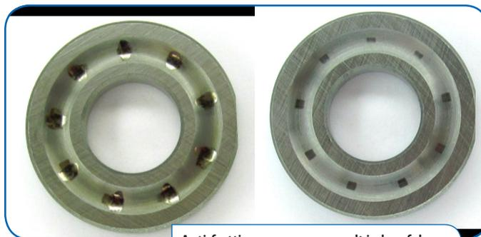
Anti-fretting grease can result in less false-brinelling wear compared to a typical EP grease when tested under ASTM D4170.
