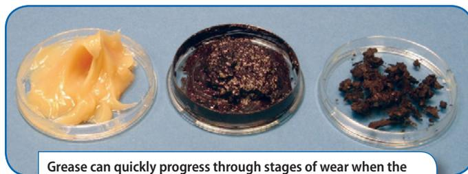
Grease can quickly progress through stages of wear when the formulation fails to meet bearing operating requirements—the result being an expensive repair in many cases.
