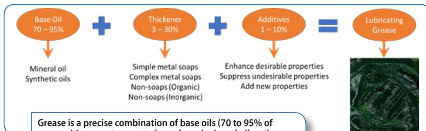
Grease is a precise combination of base oils (70 to 95% of composition; most are petroleum-based mineral oils, others are synthetic oils), thickening agents (3 to 30% of composition; agents include soaps, complexes, mixed soaps and non-soaps) and additives (1 to 10% of composition; there are many types from oxidation inhibitors to anti-wear additives).
