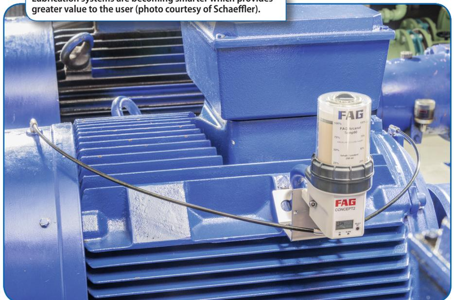
For example, Phillips said that demand lubrication based on real-time heat and vibration analysis will help drive additional efficiencies. As system recognition increases in motor amps and bearing stress indicators, it automatically increases the amount of lubrication events to manage these damaging factors through predictive maintenance.
