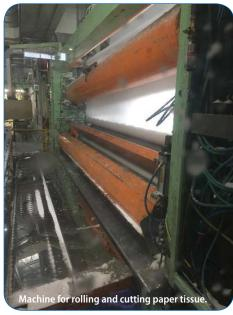
It is then separated from the feeding roll and has to be cut every 4 in. in order to fit any domestic bathroom tissue roll holders.
