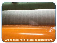
The reason why it has to be coupled and uncoupled is because space is needed for the feeding roll to feed the enrolling roll without the paper coming in contact with the cutting blades.
