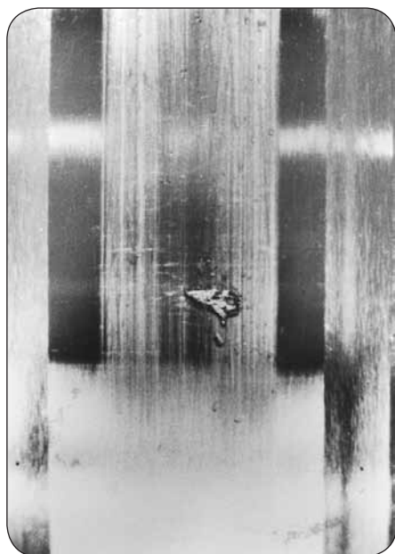
These three successive images show the fatigue progression on a bearing.
