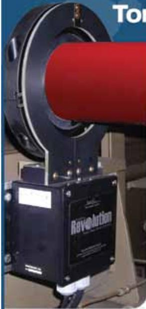
With Binsfeld systems you can do that. Whether for temporary measurements or continuous monitoring, Binsfeld telemetry instruments deliver *true mechanical* torque and power data direct from the shaft.
