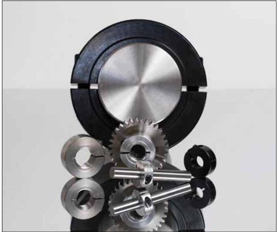
1/8" to 6" in the inch series. Clamp style shaft collars wrap around the shaft for even distribution of clamping forces. This results in a tight fit and greater holding power, without the shaft damage caused by set screws. Two-piece, clamp-style collars have an additional advantage since they can be installed on the shaft without removing other components. Ruland uses forged socket hardware in all its shaft collars, which allows for higher screw torque and increased holding power. All Ruland
