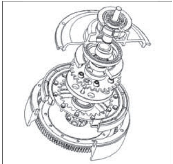
Figure 2—Sectional exploded view of Ikona CVT clutch.
