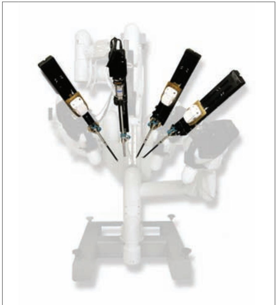
Intuitive’s “Fourth Arm” is an integral part of its da Vinci system. The first two arms represent the surgeon’s left and right hand and hold the surgical instruments. The third arm positions the 3D imaging scope, and an optional fourth arm is for adding an additional surgical instrument, effectively giving the surgeon three hands to work with. (Source: Intuitive Surgical.)
