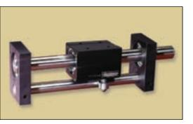
The RS indexing drive from Amacoil/Uhing provides a backlash-free alternative for linear motion systems. It comes in seven sizes to accommodate axial thrust requirements from 22 to 450 pounds. The rolling ring bearings' inner race remains in point-contact with the shaft, and between the shaft and bearings, there is no free movement. The result is that the rotary motion input converts into linear output when the shaft rotates and during reversal.
