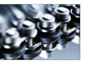
The Megalife range of power and free conveyor chains by Iwis uses a patented link with sintered metal bushes and running rollers to provide maintenancefree operation. The chain links and running rollers are supplied with a lubricant while running by a built-in lubricant reservoir. The sintered bushes are soaked in oil in vacuum conditions while the chain surfaces remain free of lubricant.
