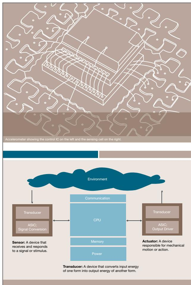
for is the creation of miniaturized devices on a chip,” he says, “so some of the key features of MEMS are small size (miniaturization), lower power consumption, and integration of electronics with sensors. So rather than having bulky external electronics, you can integrate the amplification and signal conditioning with the sensor element.”
