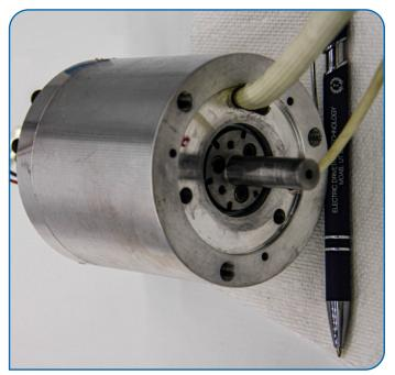
4 Nm VSR => A 75 mm diameter Switched Reluctance Motor that will deliver 8 Nm peak torque.
