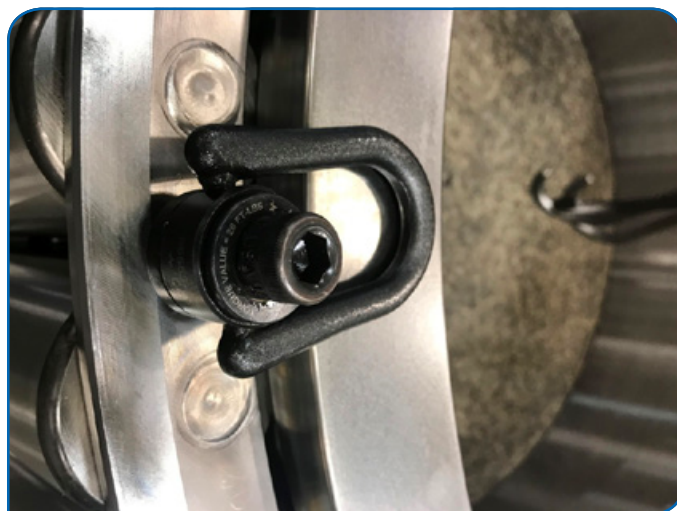
Figure 1 Tapped or threaded holes in bearing faces allow attachment devices for safe, easy lifting.
