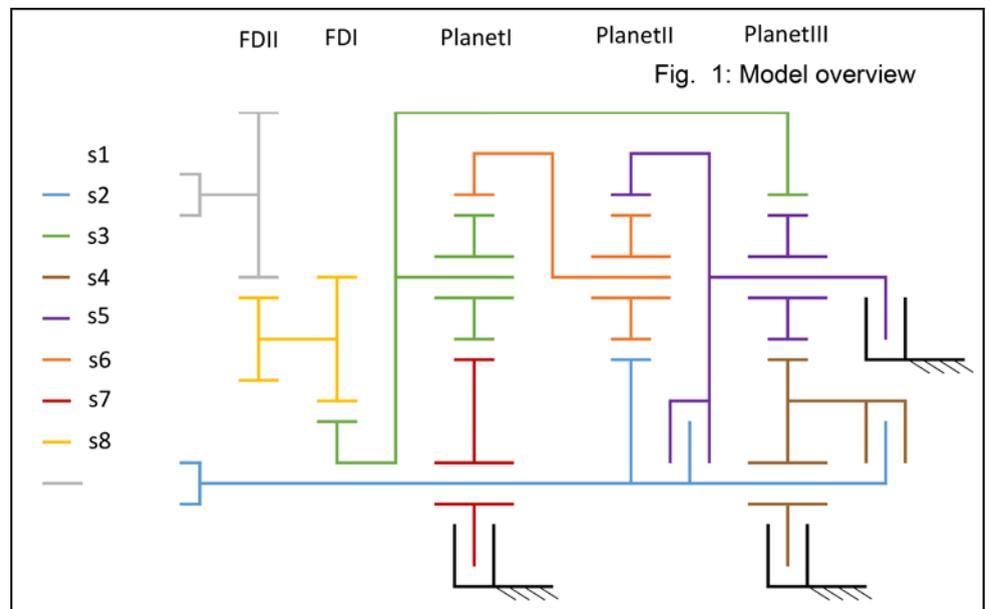
Figure 2 Shafts definition.
