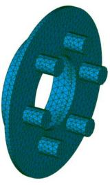
Figure 5 Carrier mesh s2.
