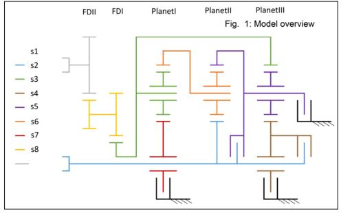
Figure 2 Shafts definition.
