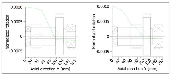
Figure 4 Influence of loads positions, example of torsion mode shape.
