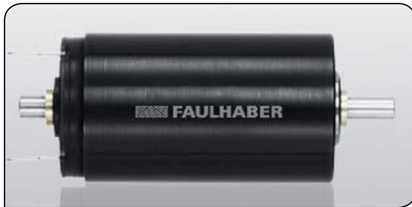
Figure 4 The graphite-commutated motor 3257 of the CR series or the 2224 of the SR series with precious-metal commutation can be equipped with radial pins to secure the suspension and to absorb the forces that arise during overload (courtesy of Faulhaber).
