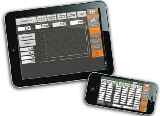
The SOBO iQ main menu allows users to access all control functions including startup, brake ramps, parking, hpU and diagnostics. The state-of-the-art SOBO iQ combines various cutting-edge technologies to provide significant flexibility, safety and durability on mine conveyors and other heavy-duty industrial applications.
