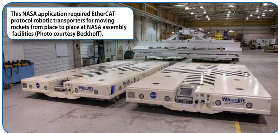
This NASA application required EtherCAT-protocol robotic transporters for moving rockets from place to place at NASA assembly facilities (Photo courtesy Beckhoff).
