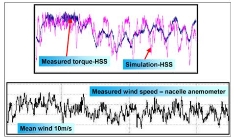
Figure 9 Comparison between a measured and simulated torque moment on the high-speed shaft of the gearbox; they are based on the same measured wind speed.
