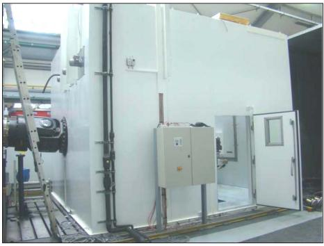
Figure 3 Eickhoff 5MW test rig with climate chamber.
