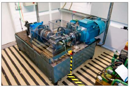
Figure 1 Electrically braced test rig at FZG.
