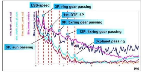
Figure 8 Comparison of frequencies included in stress signal of tower torsion based on measured and simulated data frequencies are derived from time signal of tower stress in upper-third of the tower by a fast Fourier transformation approach.
