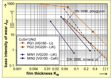
Figure 7 Base intensity of wear — all greases.
