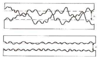
New bearing vs. broken-in bearing.
