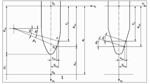
Figure 4 C and K profiles grinding wheel parameters.
