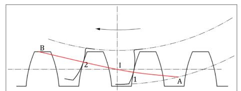
Figure 6 Active path of contact AB.
