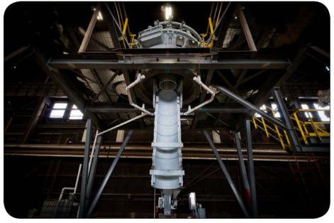
As the chute rotates through 360°, the chute is lifted and lowered by the Rexroth hydraulics to precise endpoints, as tons of iron ore and coke pellets pour down the chute into the molten iron in the furnace.
