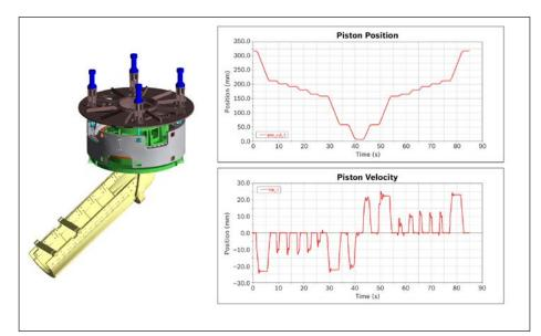
Figure 2 MOSIHS charts depicting the piston position versus piston velocity during 90-second distributor duty cycle.
