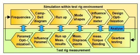
Figure 5 Coherences between influence parameters and design loop; analysis of test and simulation within optimization loop.
