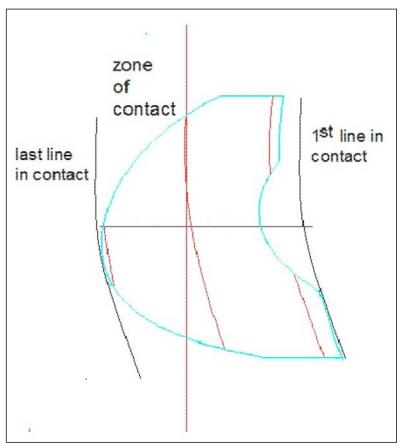
Figure 10 Contact ratio.
