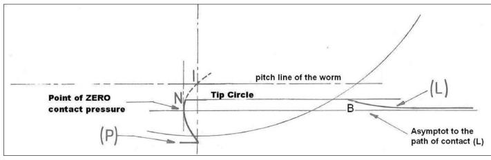
Figure 8 Limitation of gear mesh by the point of zero contact pressure angle.
