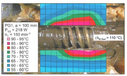
Figure 2 Heat gradient inside gearbox at worm section.
