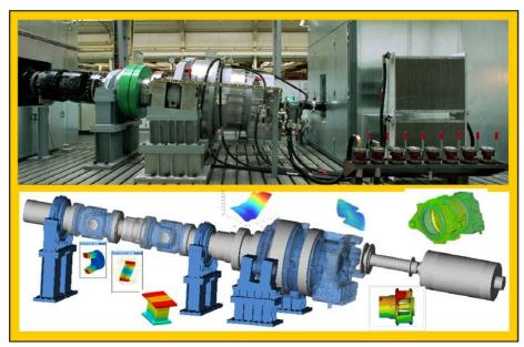
Figure 2 Photograph and simulation basis for 5 MW Wind turbine test rig; MBS (multi-body system) of the gearbox within the test rig environment.
