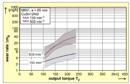
Figure 5 Wear rate for grease MIN1.
