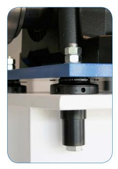
all other heavy-duty bolted joint applications. The all-spherical two-piece washer automatically adjusts under compression to compensate for up to four degrees of angular deviations. This creates an exact parallel plane between the inner face of the bolt head and inner face of the nut to distribute the load evenly over the entire inner contact surface areas. Any need for onsite machining (spot facing) to achieve parallelism is eliminated.
