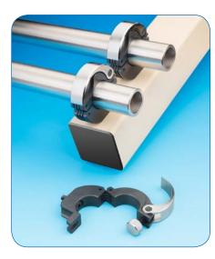
Staff-Lok Hinged Shaft Collars feature an integral hinge with a conformal cam lever for clamping and a knurled nut for adjusting the clamping preset, which makes it easy to open-close and clamp by hand. Now offered with a mounting flat with a countersunk hole and attachment screw, they are ideal for securely mounting pipe and tube requiring frequent or fast changes.
