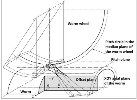
Figure 5 Pitch surfaces and offset plane.
