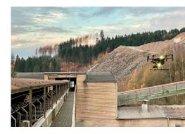
minutes, ConveyorInspect can operate over a maximum range of three miles (5 km) and at a maximum altitude of 400 ft. (130 m). The drone is equipped with a 4K Daylight Camera and 640x512 thermal camera with a frame rate of 30FPS.
