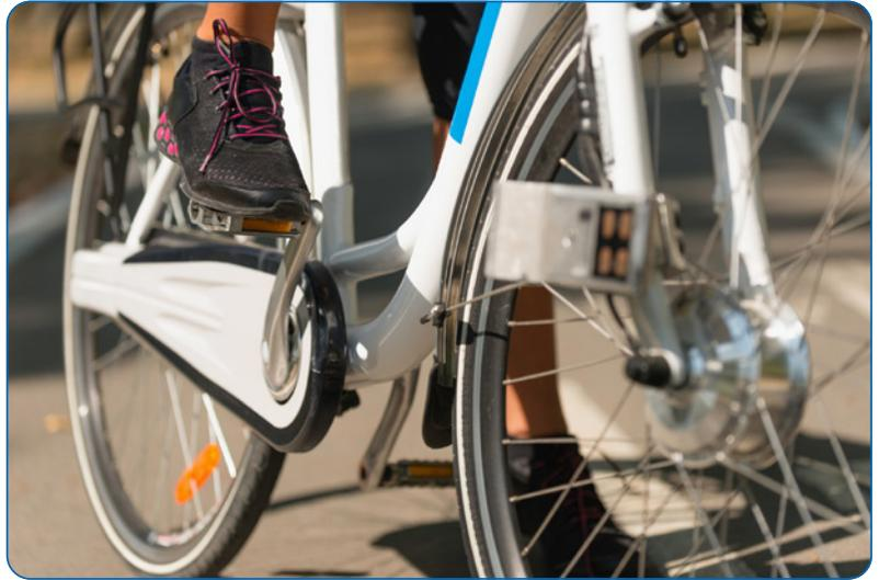
2. Light, powerful, and long-lasting electric motors. These are brushless permanent-magnet DC motors, their small size made possible by the same very powerful neodymium rare-earth magnets (10 times more powerful than Alnico) that have made recent automotive starters so tiny.
