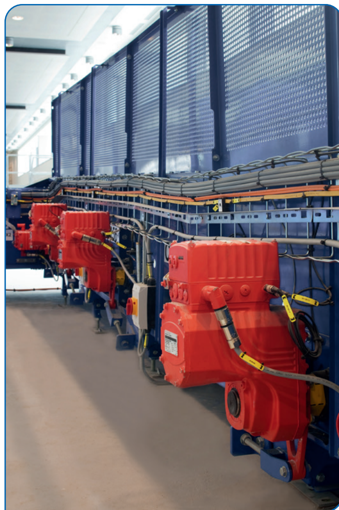
Applications that have long cable runs and multiple axes are typically the best opportunity for a decentralized control installation. Machine expansion can also be easier and less expensive. (Image courtesy SEW-Eurodrive)
