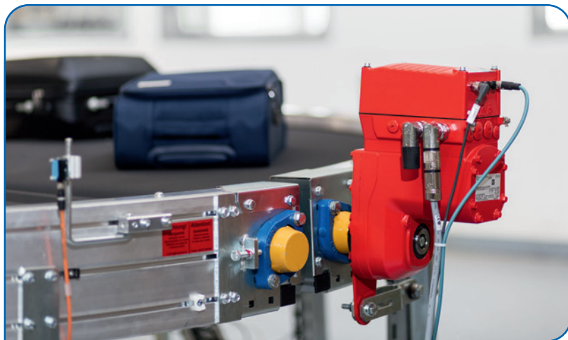
Decentralized control can include add-on components mounted on or near the motor. This modular installation can include onboard variable-frequency drives (VFDs), I/O ports, and various fieldbus options. (Image courtesy SEW-Eurodrive)
