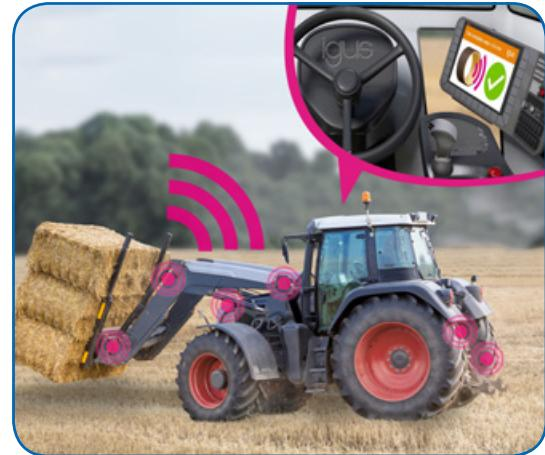
intelligent bearing detects wear and sends a signal to the user if the bearing threatens to fail. Maintenance work can therefore be planned, and operators of agricultural machines, for example, are not surprised during harvest season with an unanticipated breakdown and work stoppage.
