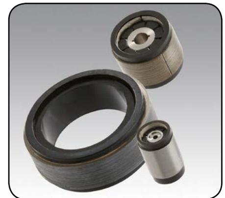
Engineered with ZeroCog slotless motor technology from Applimotion, the effects of cogging torque, magnetic forces, flux harmonics and phase balance and alignment are minimized to counteract the causes of torque ripple. Agility magnetic designs and construction techniques can achieve less than 2 percent torque ripple.
