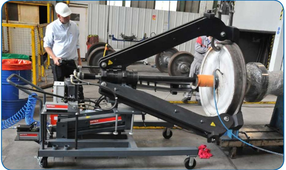
cial induction heaters can be used. Middle frequency induction heating technology is a safe and cost effective heating method that improves the quality of installation. Bega manufactures various models of the Betex MF Quick-Heater, which is also available in combination with fixed or flexible inductors.
