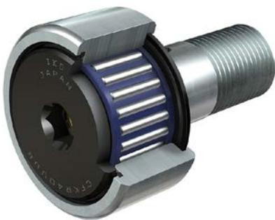
Because the structure of the CFKR series features hexagon holes on both stud ends, it can be tightened from the cam follower head or stud end. Variations are available for roller con-
