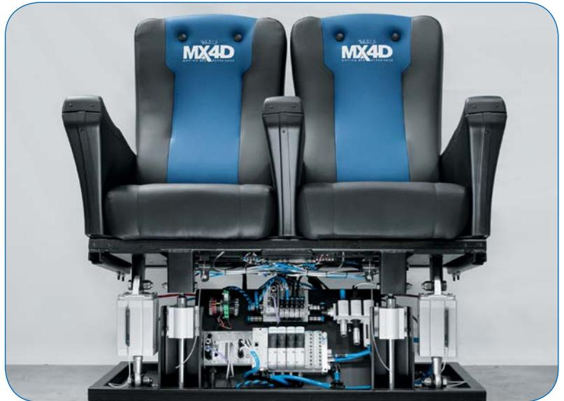
The motion profiles for the films are processed in a controller CPX-CEC directly on the Festo Motion Terminal. Many hardware components previously required are now superfluous. With the VTEM, three valves control the three actuators of each cinema seat, while one valve is responsible for pressure regulation.
