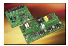
allows for accurate, variable motor speed control using Hall effect sensors for feedback. They feature a trapezoidal, two-quadrant control technique and soft start, resettable overload detection.
