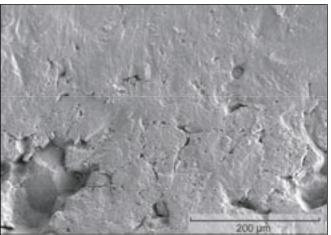
Figure 14—Surface of a 60NiTi ball after operating well beyond lubricant life of the oil. Surface shows evidence of mild abrasive wear but no galling behavior traditionally associated with titanium metallic alloys.
