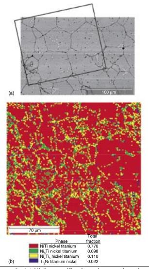
Figure 3—(a) High magnification micrograph and corresponding area image analysis (outlined box shows analyzed area). (b) Area image analyses of 60NiTi cross section showing discrete phases and their relative proportions based upon area fraction.
