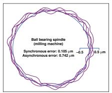
Figure 6—The ball bearing spindle shown here has more than 100 nm of synchronous error, and the asynchronous error is a large multiple (7X) of the synchronous error. This is why an air bearing spindle (Fig. 5) diamond turning or fly cutting machine can produce a mirror surface finish, while the rolling-element spindle lathe or milling machine cannot.
