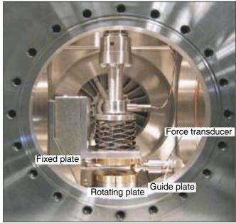
Figure 6—Spiral orbit tribometer (SOT) used to evaluate the relative lubricant life of various alloys under simulated bearing conditions.
