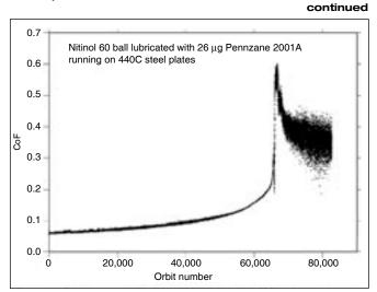
Figure 13—Friction trace of a Pennzane P2001A/Nitinol 60/440C steel system running in vacuum and continued until failure.
