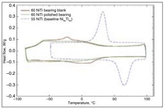
Figure 4—DSC behavior of the bearing blank material (in the softened condition) before heat treatment, and hardened and polished 60NiTi bearing ball material shown in comparison to conventional 55NiTi shape memory alloy. As expected, the 60NiTi specimens tested in this study exhibit little phase transition behavior.
