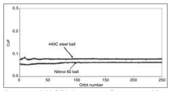
Figure 12—Initial friction traces of a system with a 440C steel ball and a Nitinol 60 ball. Both balls have been lubricated with  $\sim$  25  $\mu$ g Pennzane.
