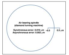
Figure 5—The difference between fluid film spindles and rolling element spindles is intuitively obvious when compared in error-motion polar plots (see also Figure 6). Notice that the air bearing spindle shown here has synchronous error of only 10 nm, and asynchronous error is a small fraction of that.
