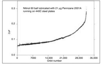
Figure 11—Friction trace of a Pennzane P2001A/Nitinol 60/440C steel system running in a vacuum.
