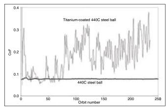
Figure 10—Friction traces of a system with a 440C steel ball and a 440C steel ball coated with a thin film of titanium. Both balls have been lubricated with ~ 25  $\mu$ g of Pennzane oil and run on 440C steel plates.
