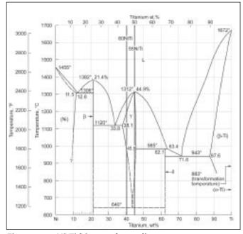
Figure 16-Ni-Ti binary phase diagram.
