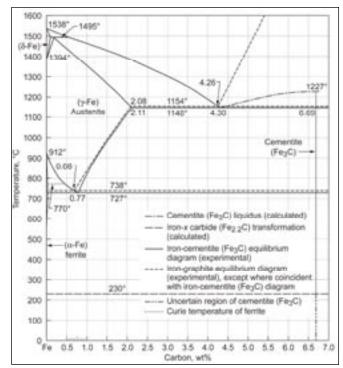
Figure 15—Fe-C binary phase diagram.
