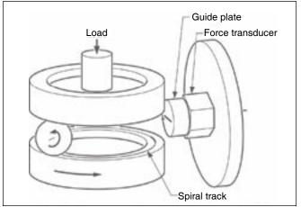
Figure 7—Components of the spiral orbit tribometer. The top plate and guide plate are stationary while the bottom plate rotates to drive the ball.
