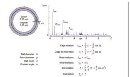
Figure 8—The above illustrates equations for calculating errors based on the relative size and number of constituent elements. A typical error motion polar plot, top left; and an FFT plot showing frequency spikes of critical elements, top right (courtesy of Dr. Eric R. Marsh).
