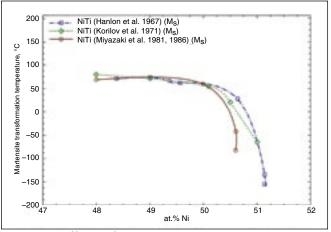
Figure 5—Effects of Ni-Ti ratio on the martensitic transition temperature demonstrating that at high Ni-contents, the martensitic transformation is suppressed to very low temperatures. This implies high dimensional stability for the 60NiTi alloy.
