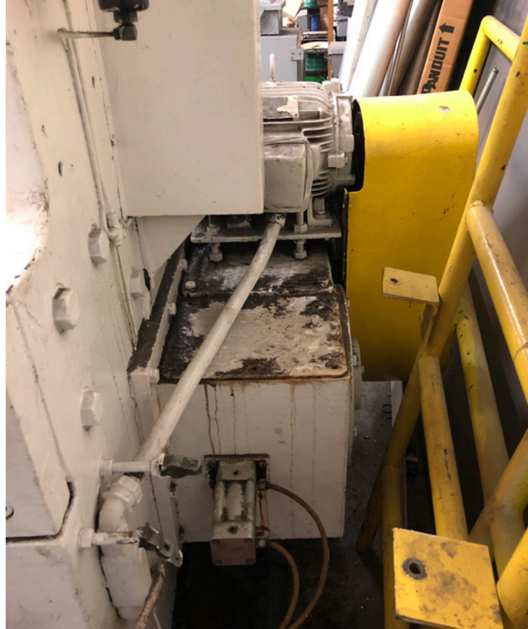
Old design with original clutch brake.
